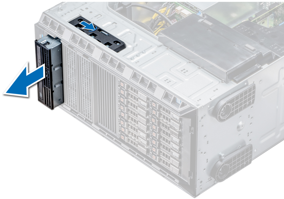
Figure 40. Removing the optical drive cage or tape drive
